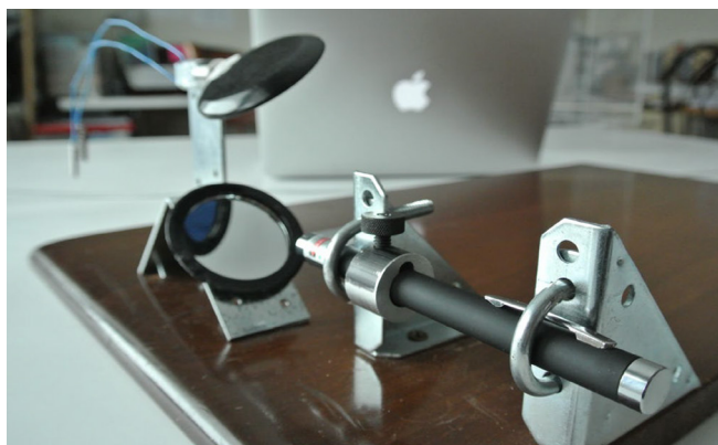
FIGURE 6. Laser-scanning fuel-spray visualizer with motored rotating mirror used for spray-pattern measurements
