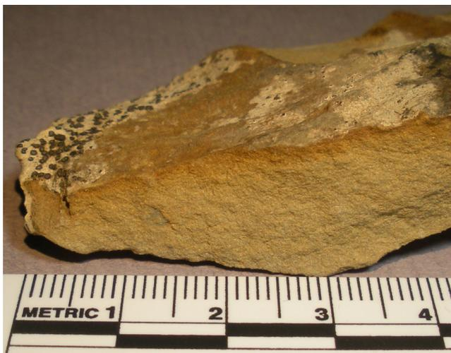
FIGURE 8. Photograph of brown Buena Vista Member, sample CMNH 8963, broken normal to the weathered surface showing the depth of brown iron oxide weathering.
