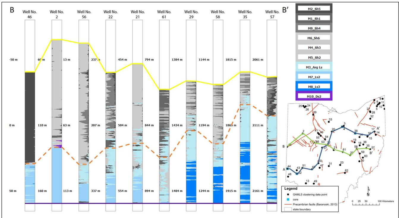
FIGURE 10. Cross-section B-B’ trending west to east. The yellow line marks the top of the Point Pleasant and Utica shales; the brown dashed line marks the approximate top of the Trenton and Lexington limestones; and the purple line is the datum, marking the top of the Black River Group. Modes are numbered and color-coded to reflect the same lithofacies interpreted in Table 2. Depths are relative to sea level.
