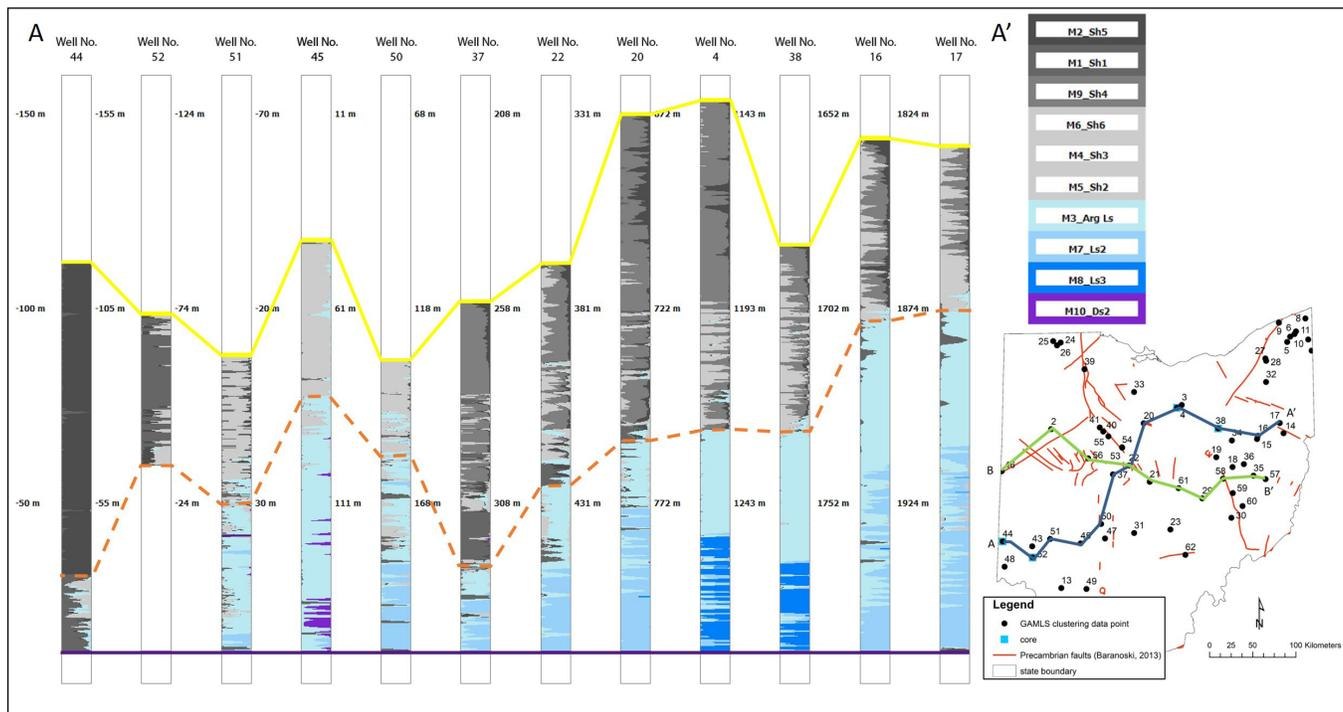
**FIGURE 9.** Cross-Section A-A' trending southwest to northeast. The yellow line marks the top of the Point Pleasant and Utica shales; the brown dashed line marks the approximate top of the Trenton and Lexington limestones; and the purple line is the datum, marking the top of the Black River Group. Modes are numbered and color-coded to reflect the lithofacies interpreted in Table 2. Depths are relative to sea level.
