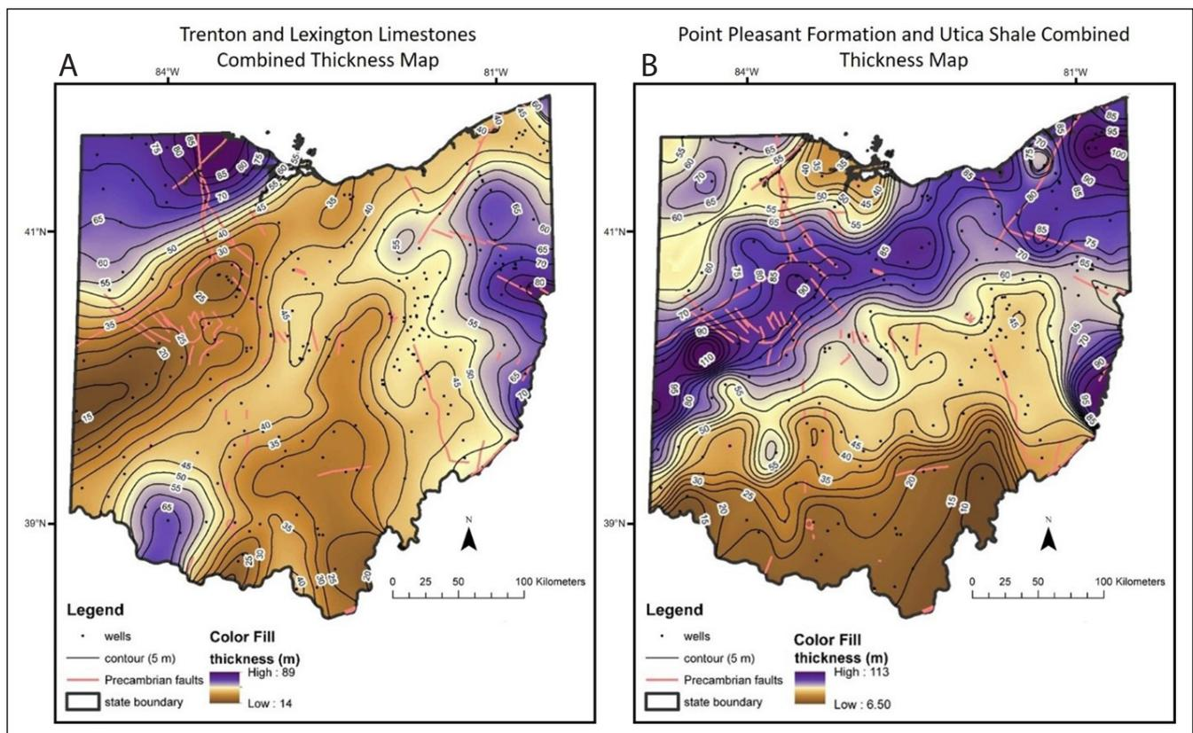
**FIGURE 8.** Isopach maps for (A) the combined Trenton and Lexington limestones, showing noticeable thinning from southwestern through northeastern Ohio, and (B) for shales in the overlying Point Pleasant Formation and Utica shale, which exhibit noticeable thickening along the same southwest-to-northeast trend in Ohio. These thinning of the limestones and thickening of the overlying shale units suggest an extension of the Sebree Trough throughout northeastern Ohio (see Figs. 2B, 3, and 4).
