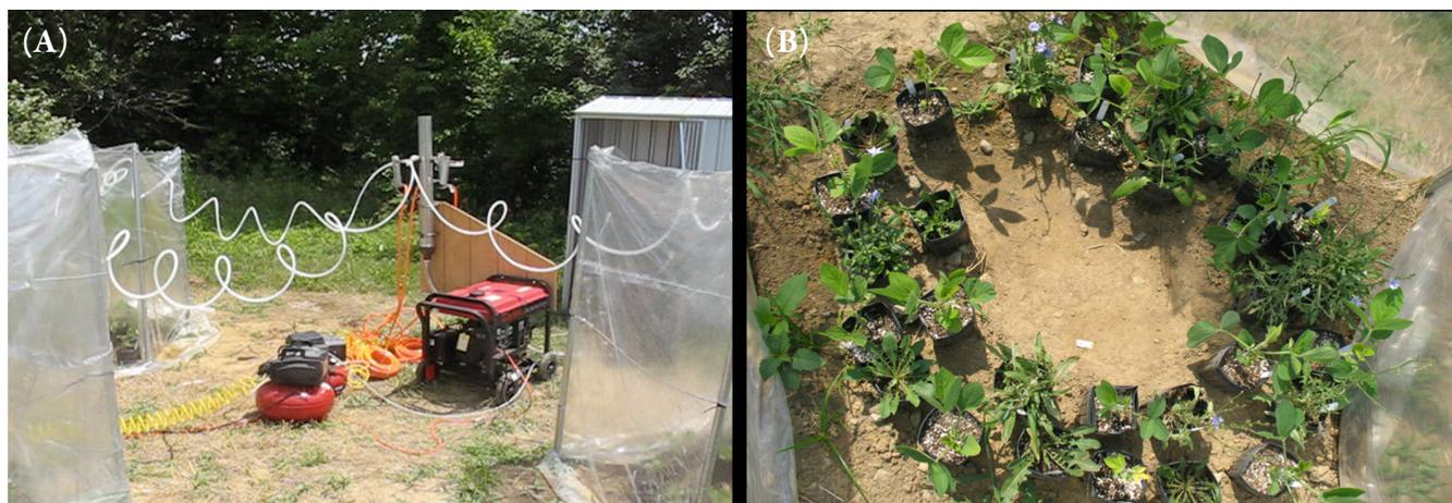
FIGURE 1. Experimental design detailing (A) the generator with exhaust manifold and air compressors used to distribute diesel exhaust to individual chambers and (B) arrangement of soybean (*Glycine max*) and chicory (*Cichorium intybus*) plants within an individual chamber. Fifteen potted plants of each species were alternatingly planted in 2 circles around a central drainage point.
