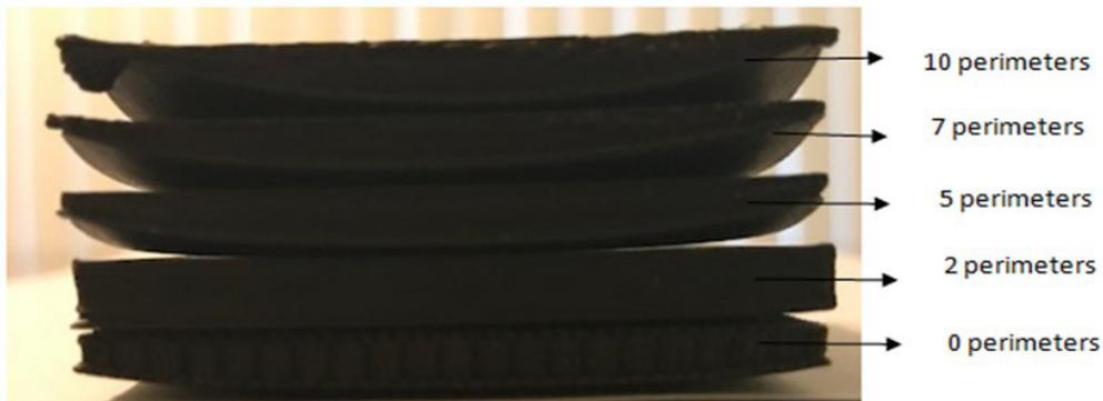
FIGURE 6. Sample thickness profiles corresponding to 0, 2, 5, 7, and 10 perimeters
