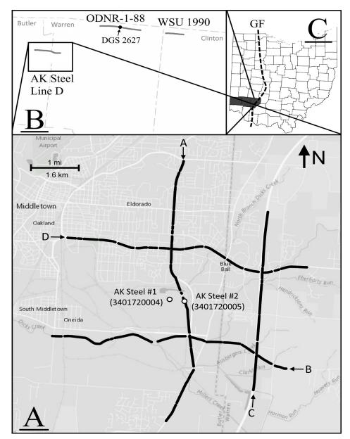
FIGURE 1. (A) Locations of the AK Steel Seismic Lines A, B, C, and D, and AK Steel #1 and #2 boreholes (name and API#) at Middletown, Ohio. Arrows indicate the increasing shot directions. (B) Regional relationship of Seismic Lines ODNR-1-88, WSU 1990, and core hole DGS 2627 to the AK Steel study area with Seismic Line D. (C) Ohio county map showing the Grenville Front (GF) (dashed line) after Kim et al. (2000).
