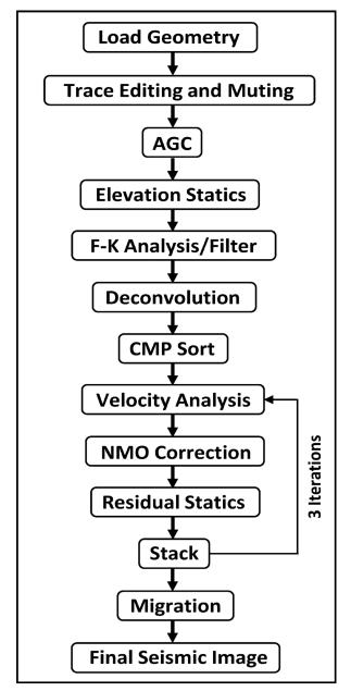
FIGURE 2. Flowchart of steps employed to reprocess all 4 of the AK Steel seismic lines. Note that 3 iterations of velocity analysis and residual statics were performed.
